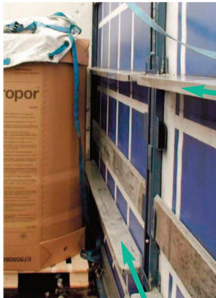
Picture 4: Typical turnable side bars and a typical octabin load; turnable side bars may be used to avoid airbags and other materials to fill up empty lateral space on the loading platform.
