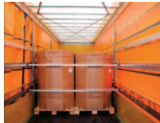
Picture 3: Examples for different load securing systems using form-lock securing
