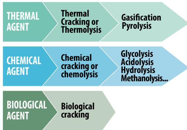
**Thermal cracking (Thermolysis).** The polymer chain is broken using temperature and, in some cases, catalysts. The main processes or techniques are **pyrolysis** (carried out in the absence of oxygen) and **gasification** (with oxygen). Generally, thermolysis takes place under more stringent conditions than total combustion. It is applicable to waste composed of both addition and condensation polymers.
