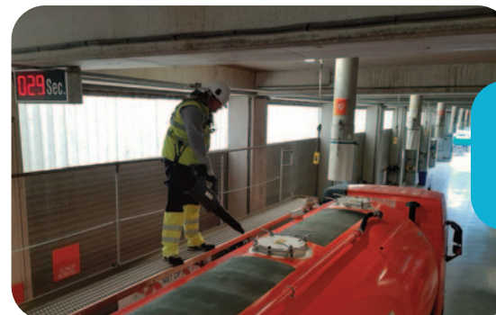
Manual cleaning after bulk loading
